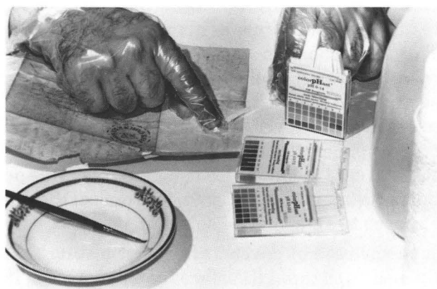
Figure 30. PH testing with ColorpHast® Indicator Sticks. The test sticks always should be stored in a clean, dry area away from any chemicals in order to ensure their accuracy.
