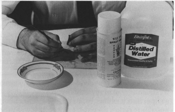
Figure 5. Testing for ink stability: applying solution.
