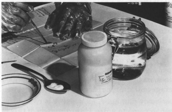
Figure 12. Reduction of stains using Chloramine-T. A fresh solution of Chloramine-T should be made before every treatment session.
