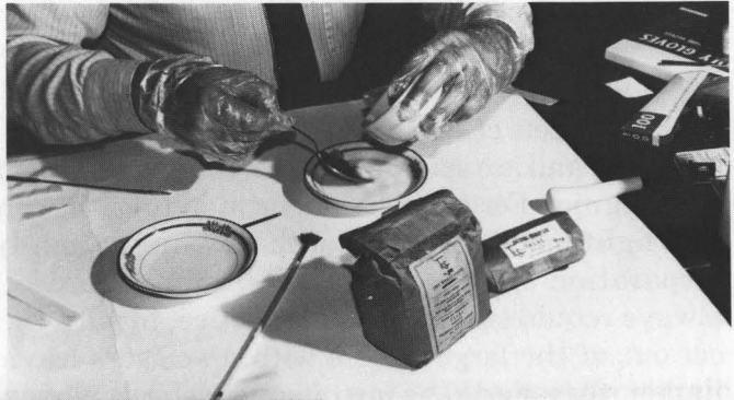
Figure 20. Preparing wheat paste. Smooth paste of the consistency of thick cream is prepared fresh before every treatment session.
